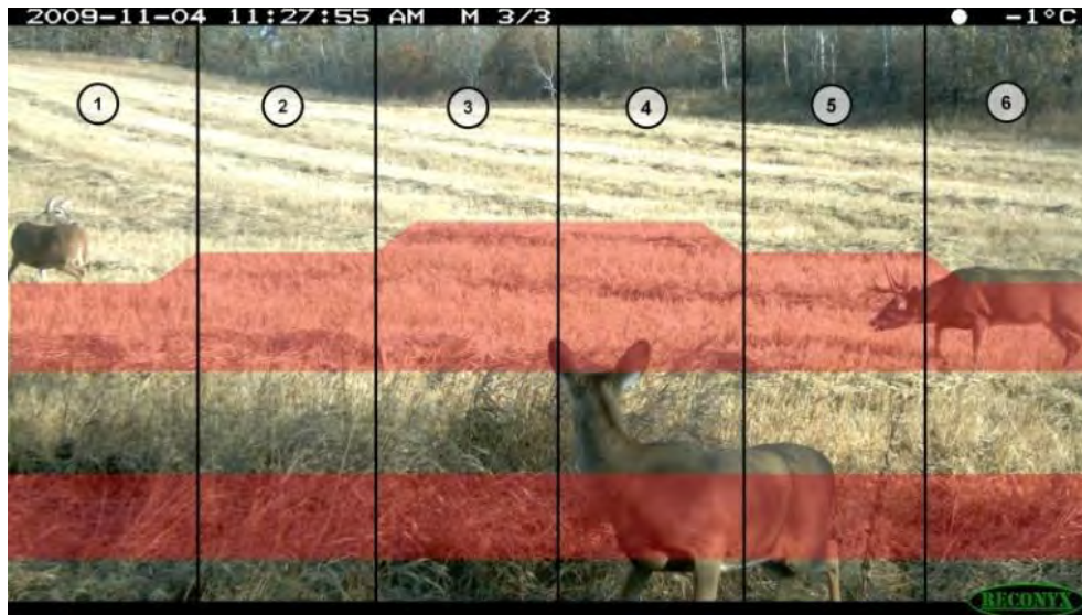
Figure 7. The detection zone in a Reconyx HC500, HC600 and HC800 camera trap showing the warm zones (noted by pink) and sectors where animals have to cross to trigger a photo. The deer in sector 1 would not have triggered the camera (image: Reconyx).
