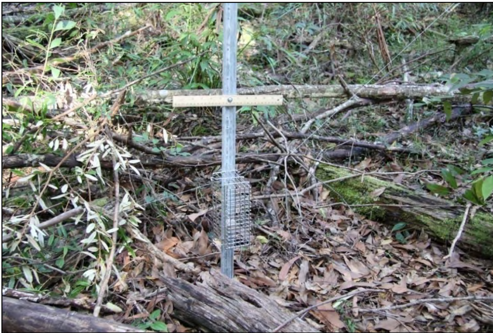
Figure 20. An example of a method for maintaining food lures used in northern NSW. A tea infuser containing bait is wired behind a cutlery drainer and suspended on a steel picket. The ruler can be fixed to the picket to assist with image scaling. By suspending the tea strainer inside the cutlery drainer the setup not only excludes small- and medium-sized mammals but ants too (image: Paul Meek).
