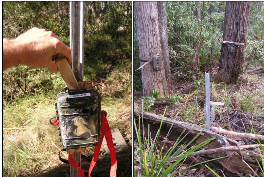
Figure 14. Attachment of cameras using wedges and sticks to aim the camera directly at the focal point (image: Paul Meek).
