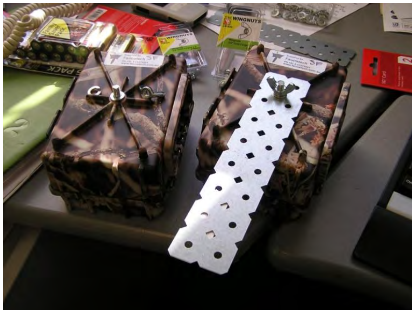
Figure 19. This generic bracket can be attached to camera traps that have tripod fittings and screwed into trees or fastened with bolts to posts. Similarly, lengths of steel strap bracing, cut to length, can be used as a more flexible substitute. In either case, a short piece of threaded rod is used with wing nuts to secure the device (image: Paul Meek).
