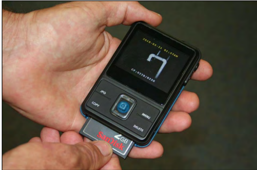
Figure 13. The Cudviewer (or similar device) allows you to view images taken by cameras that use SD cards and compact flash cards (image: Paul Meek).
