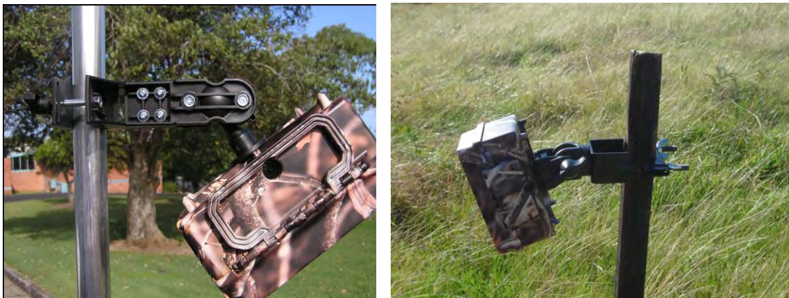
Figure 18. Outdoor camera mounting bracket and Reconyx steel-post fitting for attaching camera traps to pickets and posts (image: Paul Meek).
