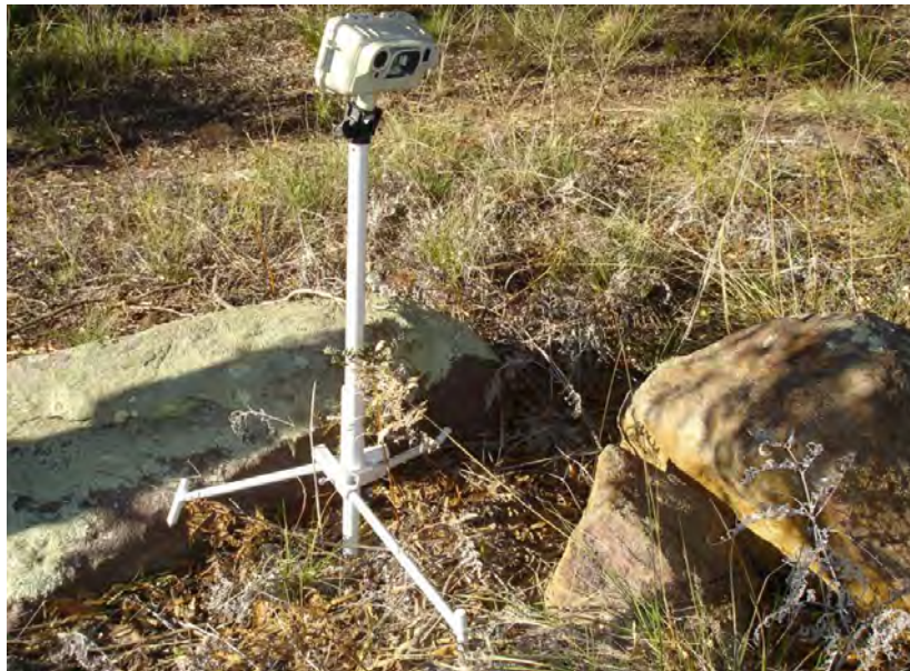
Figure 16. The Faunatech Rockpod is a sturdy and adaptable tripod-type device (image: Ross Meggs).
