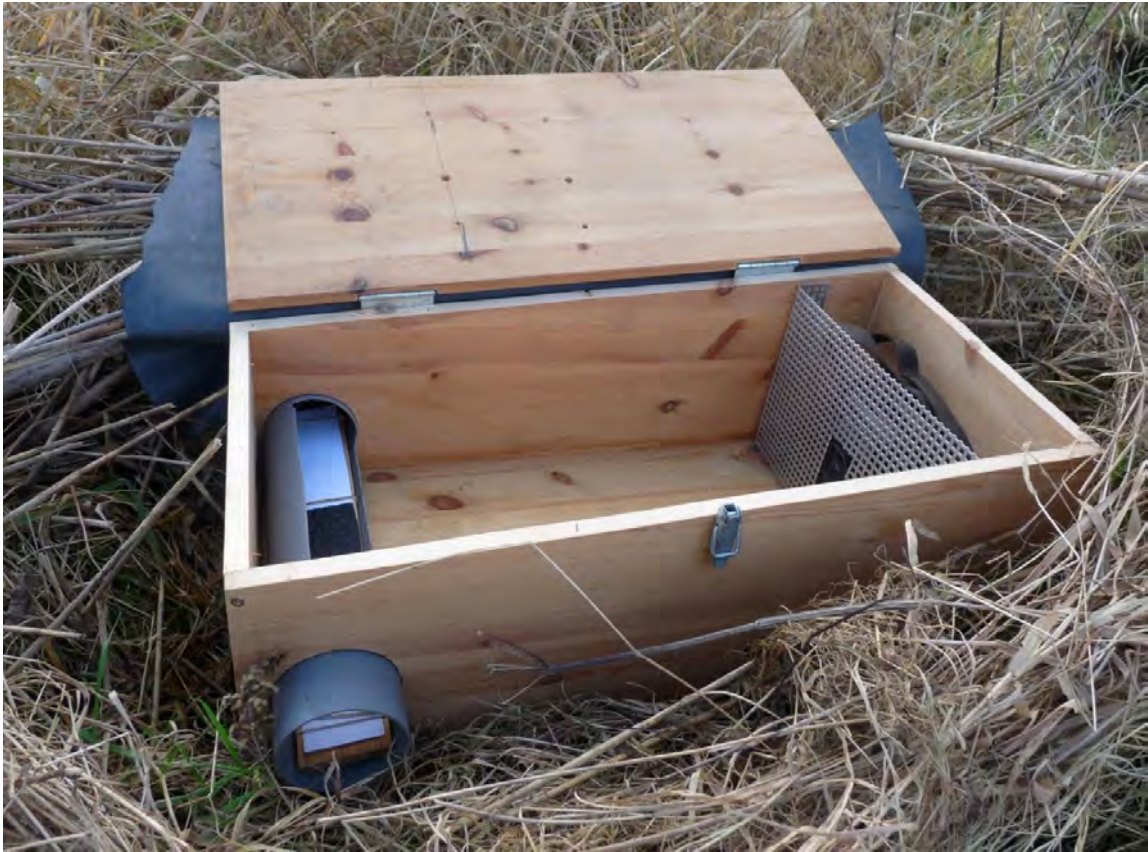
Figure 30. The ‘Mostela’ device for capturing images of fast moving mustelids such as weasels (image: Jeroen Mos).
