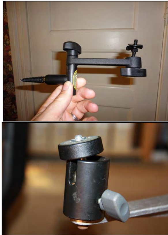
Figure 17. Ezi-Aim screw (top) camera trap mounting device for trees and a tripod-type mounting bracket design (bottom) by KORA (image: Paul Meek).
