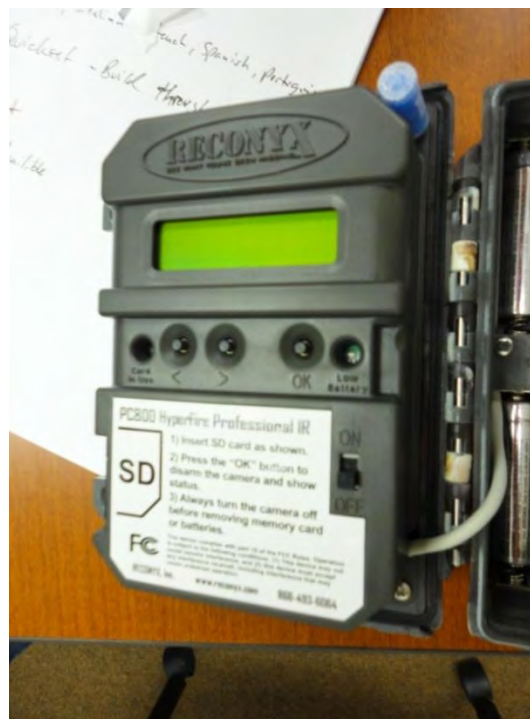
Figure 11. Finding a place to deploy moisture desiccant can be challenging. The best location in a Reconyx camera where a canister can be used is in the corner of the housing (image: Paul Meek).
